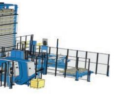
The large Night Train system automates the material and information systems of the factory's cutting and punching operations, combining individual manufacturing steps into one process. It features over 400 storage drawers.
